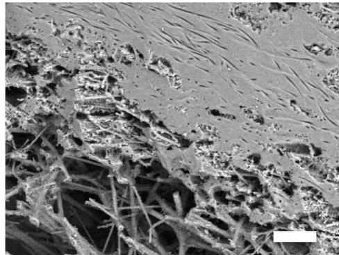
*Figure 2. SEM image of silica precipitates around bacterial filaments from an alkaline hot spring in Yellowstone showing a transition from individual bacterial filaments coated with silica (bottom) to massive infill of microbial filamentous biofilm (top). Scale bar is 20  $\mu\text{m}$ .*
